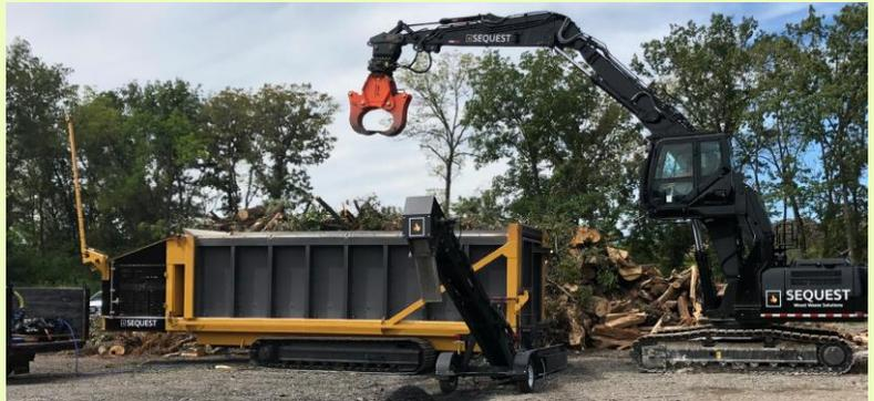
The Carbonator 500 is a mobile biochar production system that converts trees, brush, stumps and other wood debris into a high-quality biochar. At nearly forty feet long, the immense Carbonator 500 is capable of burning 15-20 tons of wood waster per hour, with five to ten percent of the material converted into biochar.
